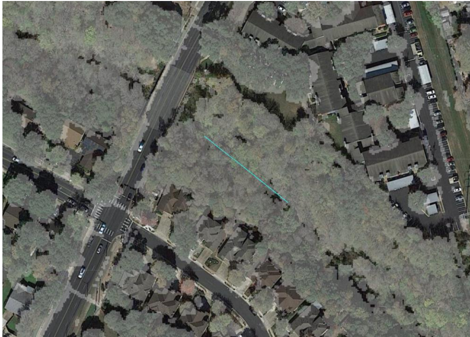
Figure 7 Image showing the accuracy of how the LPC dedicates land area as vegetation. The transparent light gray overlay represents the vegetated area. The line in blue shows where the buffer line was drawn for this station location.
