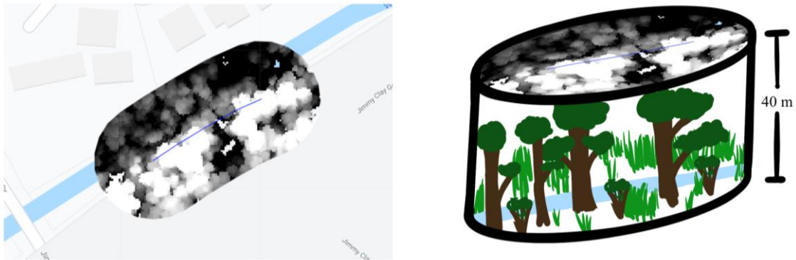
Figure 8. Visual of the process used to extract the volume of vegetation on a streambank. The sum of all the heights of each 1x1 meter vegetation pixel (high, medium, and low) are multiplied by the area of the buffer to get a volume of vegetation. This volume is then divided by the total volume of the initial volume (bank area x 40 m) to get a percent volume of vegetation.
