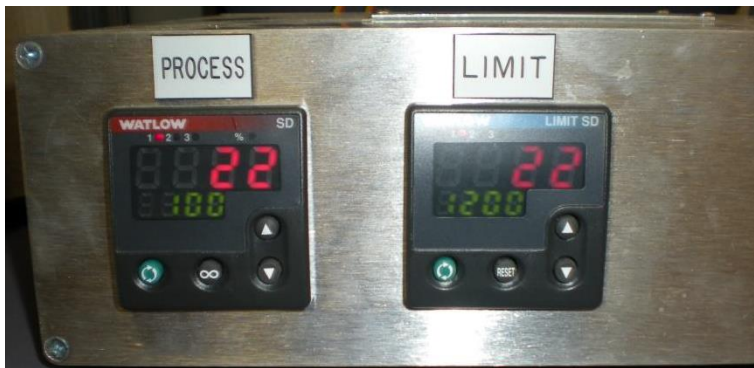
Figure [8]. Temperature controller displays. The target set point is controlled by the process display
