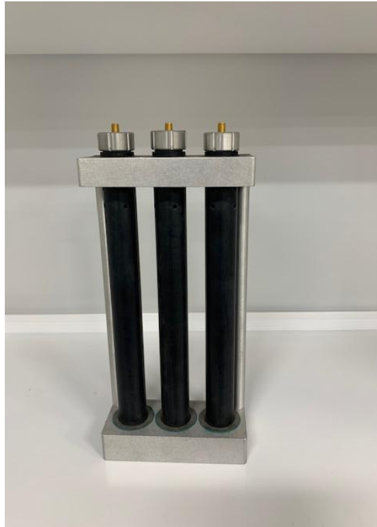
Figure [5]. Set up of sapphire rods on to the transducers
