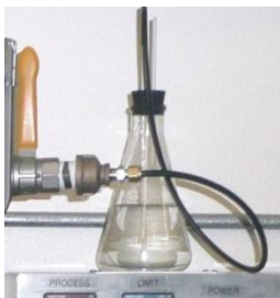
Figure [7]. Bubbler to control flow of inert gas
