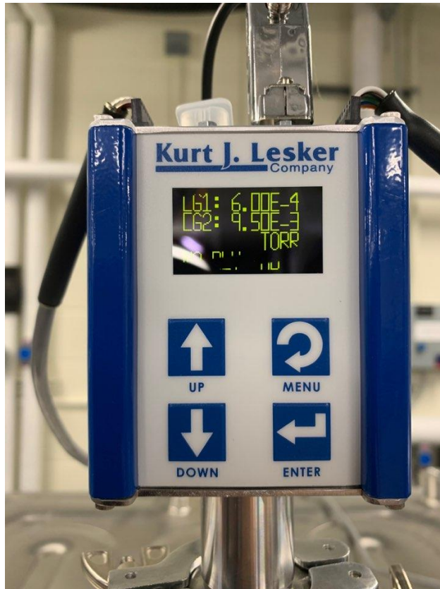
Figure 15. Vacuum gauge of pressure inside the chamber
