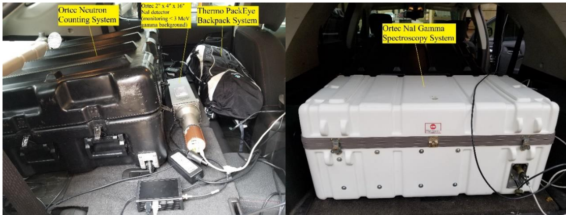
Figure 2-4. Photos displaying the detector systems' placements when mounted in an SUV-type vehicle for these measurements looking into the vehicle from the rear passenger side door (left) and the trunk (right).
