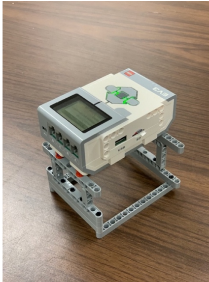
Figure 8. EV3 Intelligent Brick, showing the motor ports, PC port, USB port, and SD card port.
