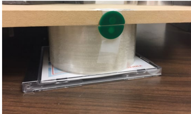
Figure 4. GM dead time determination and statistical analysis experiment in the proof-of-concept remote laboratory for radiation detection education. This is the apparatus when half-source A and half-source B are measured as a whole source (Emery, 2018).
