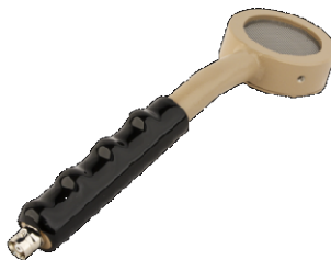
Figure 1. This is called a pancake probe because of its cylinder-like head.
