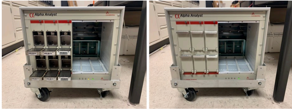
Figure 54. Apparatus of the alpha spectroscopy and attenuation experiment with chamber doors open (left) and closed (right).
