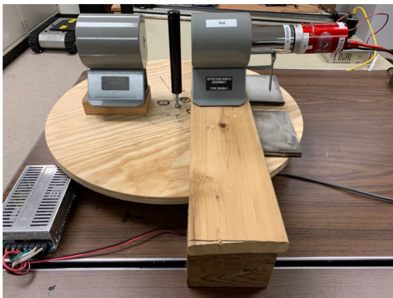
Figure 1. ^{137}\text{Cs} source placed at an angle of 0^\circ with respect to the NaI detector.
