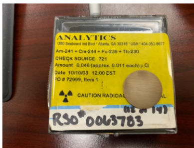
Figure 1. This is a mixed alpha source to be placed in the alpha spectrometer.
