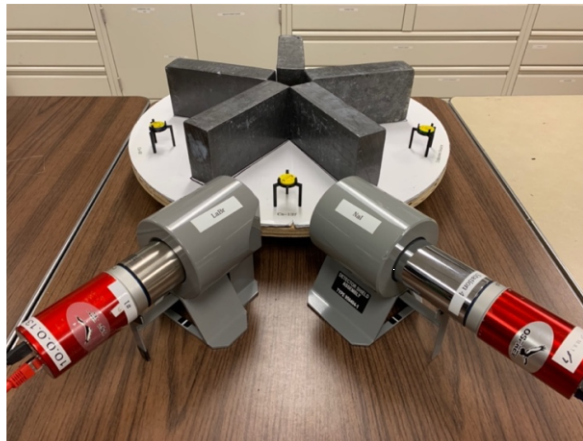
Figure 2. Experiment apparatus with LaBr on the left and NaI on the right.
