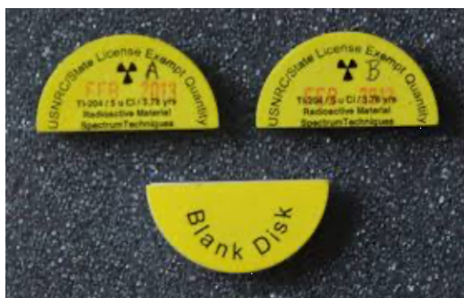
Figure 3. The “split” source has two hemispheres each containing a 5 \mu\text{Ci } ^{204}\text{Tl} when it is new. These sources have a relatively short half-life so that is not the activity today. The “Blank disk” issued to help with the placement of half-sources below a detector face. It helps maintain source-detector geometry between source change-outs.
