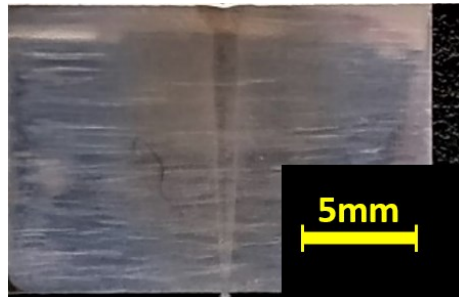
Figure 3.20 Weld transverse section of the sample A1 measured by a caliper (polished and etched)
