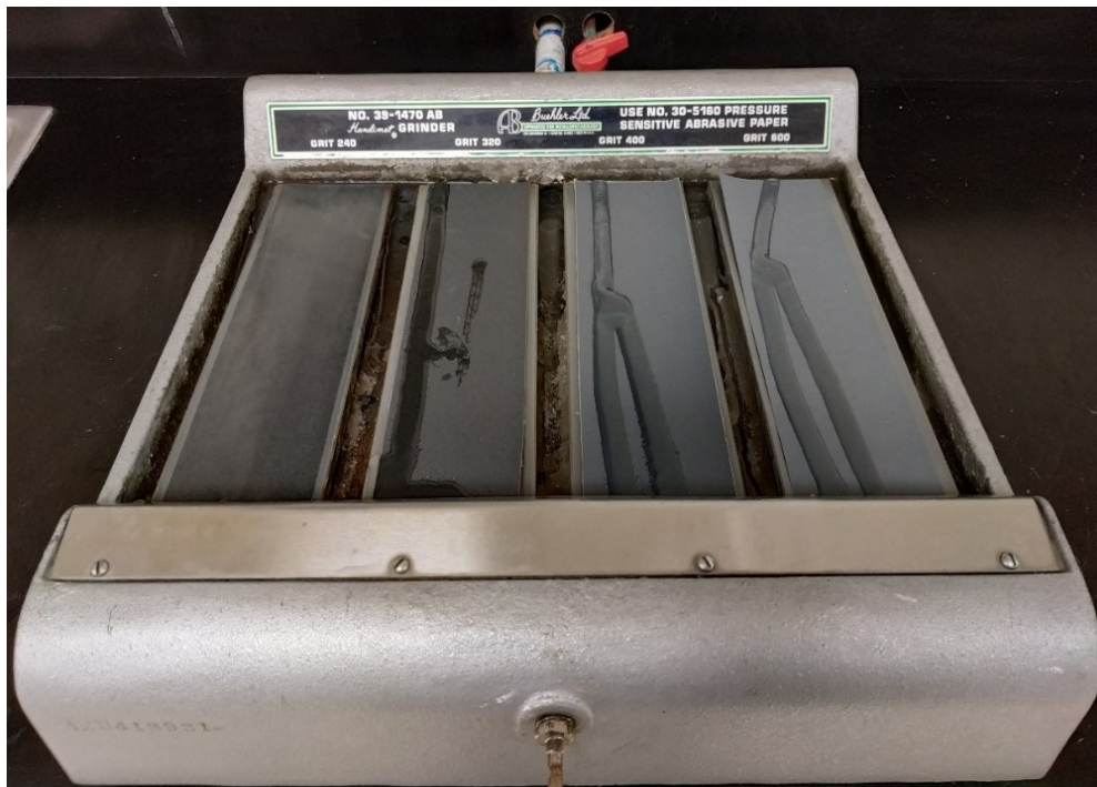
Figure 3.13 Handimet grinder with different grit size abrasive papers
