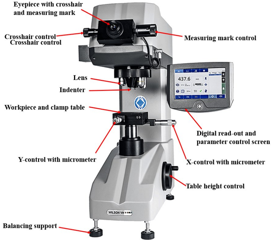
Figure 3.25 Wilson VH1102 microhardness tester (source: Buehler Materials, https://www.buehler.com/wilson-VH1102-1202-micro-hardness-tester.php )
