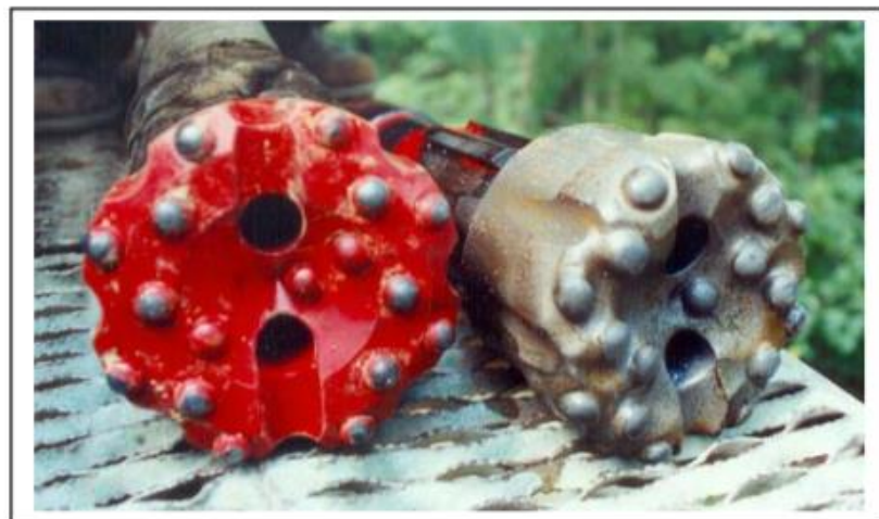
Figure 2.5 Solid-head bits for percussion drilling [11]
