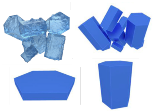
Figure 5.11: Illustration of the four ice particle habits used in the shape sensitivity study. Shown is an aggregate of severely roughened hexagonal columns (top left), aggregate of smooth hexagonal columns (top right), plate (bottom left), and single hexagonal column (bottom right).
