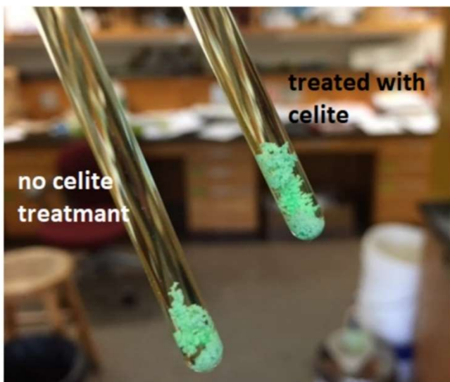
Figure 58 Precipitate formed in the reaction between ethoxyacetylene and AzCou
