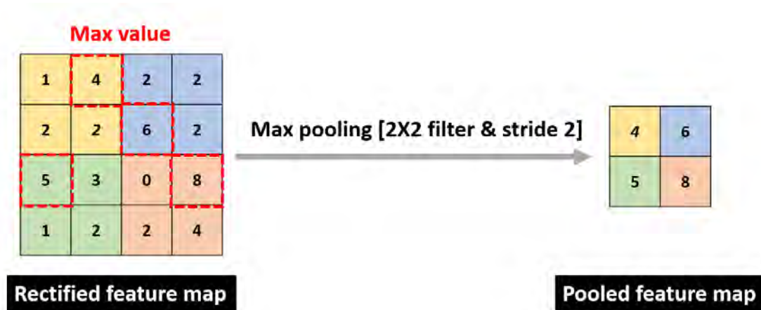
Figure 4.3: Example of max pooling operation with 4 \times 4 feature map.
