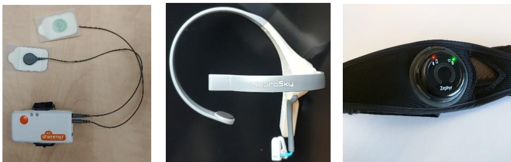
Figure 4: Physiological devices used in the study. From left to right: Shimmer GSR, NeuroSky MindWave, and Zephyr BioHarness.
