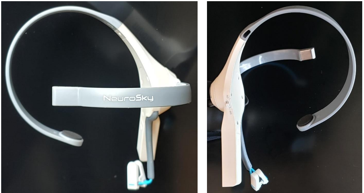
Figure 8: NeuroSky Mindwave. The figure on the left presents the front of the device; the single electrode is placed in the FP1 position is visible in the figure on the right. The clip attaches to the ear as the reference electrode.
