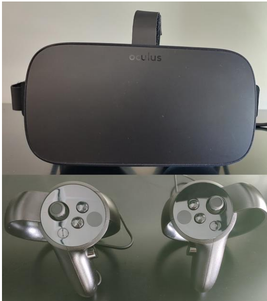
Figure 54: Oculus VR system. The headset is shown in the top figure, and the Touch controllers on the bottom figure.
