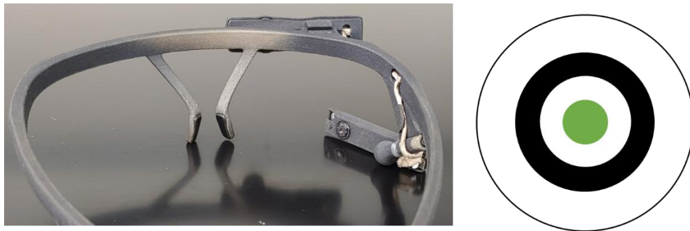
Figure 33: On the left, Pupil by pupil labs. The camera that faces the pupil is shown. On the right, is the target that was used to calibrate the Pupil.
