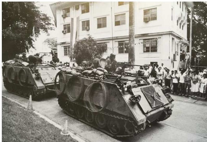
Figure 2. M113 Armored Personnel Carriers (APCs) on narrow Panamanian Streets. The vehicle commander served as the .50 cal. gunner to protect the APC and the exposed infantrymen standing in the rear troop compartment. 82
