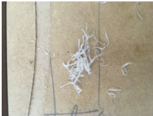
Figure 4.14: Straight line machine chips created using 3/8" bit.
