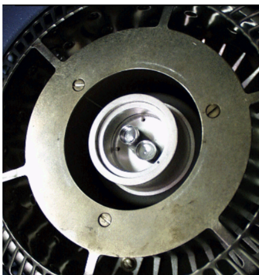
Figure 3.10: TA Instruments DSC Q2500 Cell showing the reference pan and sample pan in the cell where the heat is applied. Each pan has a thermocouple underneath it. The difference in temperature between the reference and sample thermocouple readings are recorded [9].
