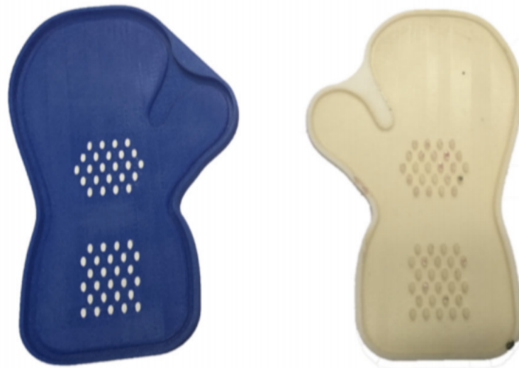
Figure 6.2: (Left) 3D Printed ABS make mold to cast silicone. (Right) Silicone Female Mold to cast SMP [20].
