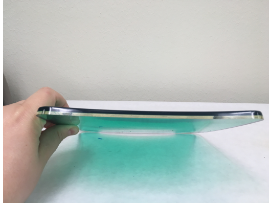
Figure 2.11: Layered SMP structure ( T_g=50-60^{\circ}\text{C} for the green layer and T_g=80-100^{\circ}\text{C} for the clear layer).
