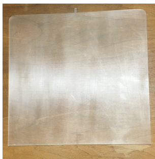
Figure 2.10: SMP sheet made using injection molding with a pressure pot.
