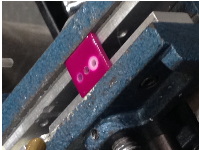
Figure 4.4: Thermochromic heat sensing during machining.
