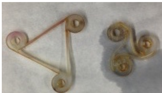
Figure 5.6: Contraction of chiral structure: expanded (left) and compressed (right) states [19].
