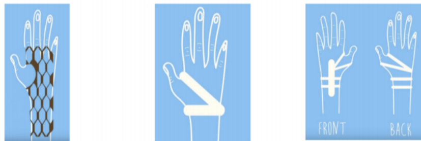
Figure 6.4: (Left) Depiction of paper prototype of honeycomb design based on Chinese finger trap. (Middle) Depiction of paper prototype of strip strap design optimized for simplicity. (Right) Depiction of paper prototype of bosani design providing maximum support with minimal material [20].
