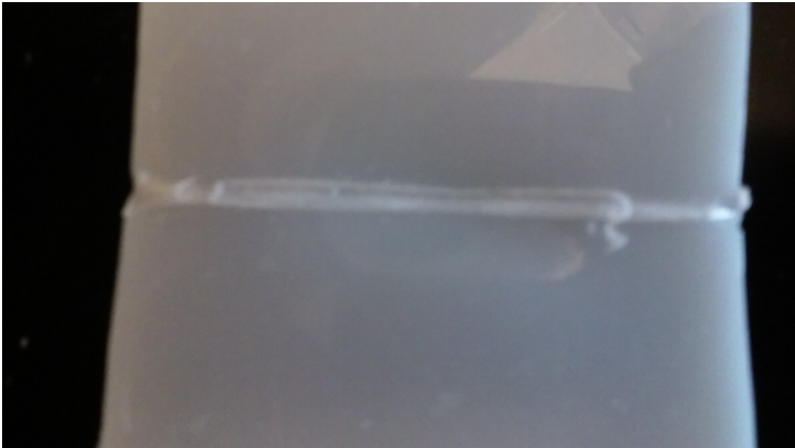
Figure 4.12: UHMWPE cut with the rounded bit. (The ends have a larger, more rounded groove, while the middle portion maintains a more uniform width and thickness.)
