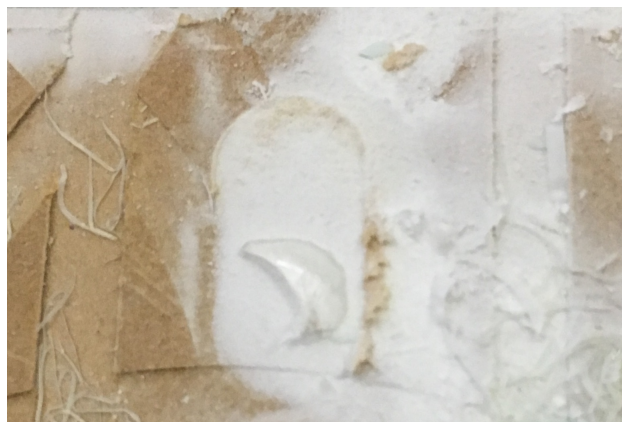
Figure 4.15: Fine powder machine chips created using 1/2" bit.
