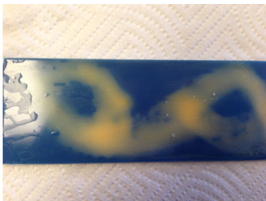
Figure 2.7: SMP with incorporated thermochromic powder and dye.
