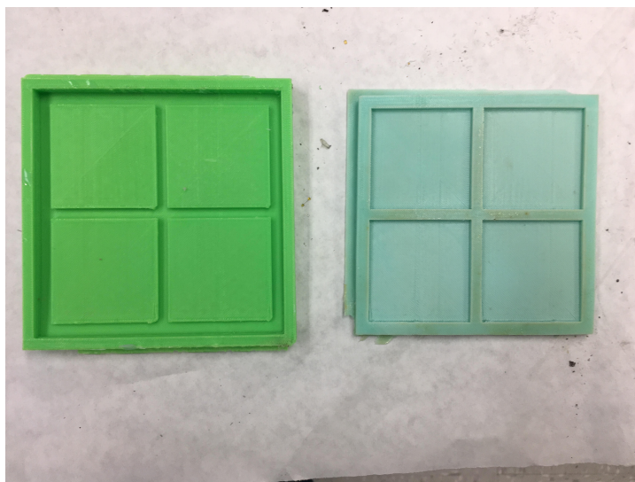
Figure 2.6: Male and female molds for casting SMP: (Left) ABS mold (Right) silicone mold.
