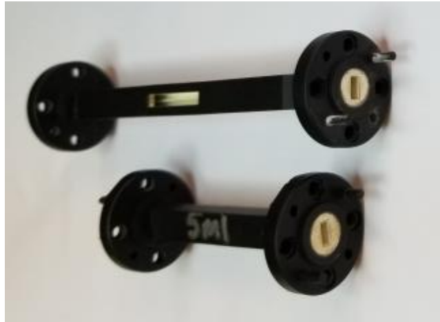
Figure 21 The metal plated 2-inch WR-15 waveguide section and trough waveguide
