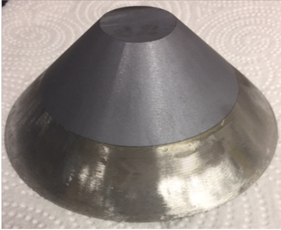
(a) Si crystal after grinding in the bevel platform
