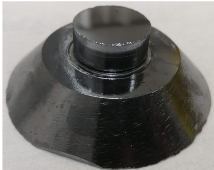
Figure 2.5: Fabricated conical detector from cylindrical Si crystal
