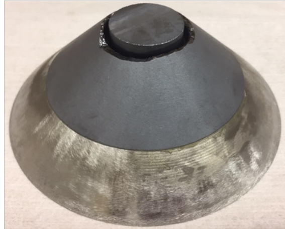
(b) Si crystal after core-drilling
