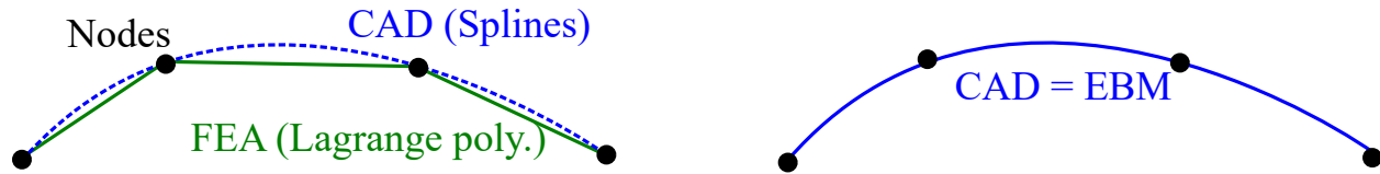
Figure 7.3: Traditional methodology vs. universal parameterization methodology, where EBM stands for Euler-Bernoulli method. A universal parameterization method enables higher accuracy analysis without approximating the topology with a mesh of low-order piecewise polynomials.
