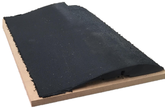
(a) 2lb XLPE machined foam core
