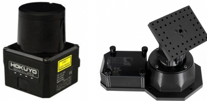
Figure 12. HOKUYO LIDAR (left) and PhantomX XL-430 robot turret(right)
