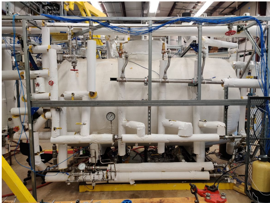
Figure 3.3. Suppression chamber analog with associated piping.
