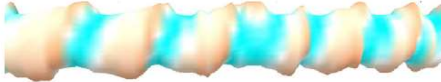
Figure 1 –Spiral hole with 3 foot pitch (period) length (Dupriest et al., 2010)
