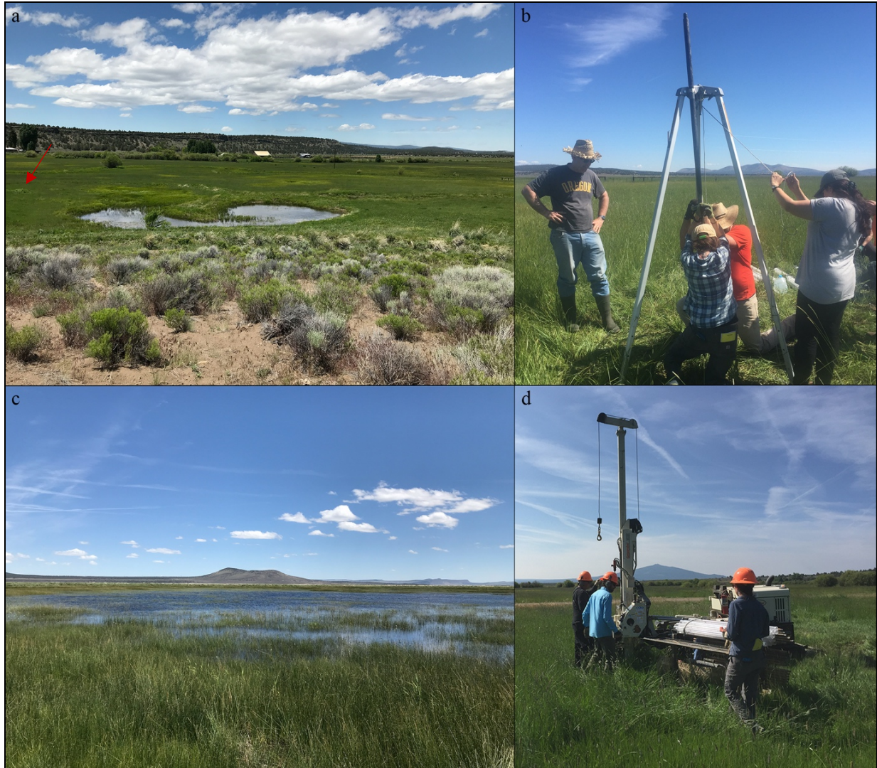
Figure 4.5. Coring in Site 2: (a) area just north of site 2A, arrow points to coring location; (b) coring with modified Livingstone in 2018; (c) view of marsh looking north-northeast; (d) coring with Geoprobe in 2019.
