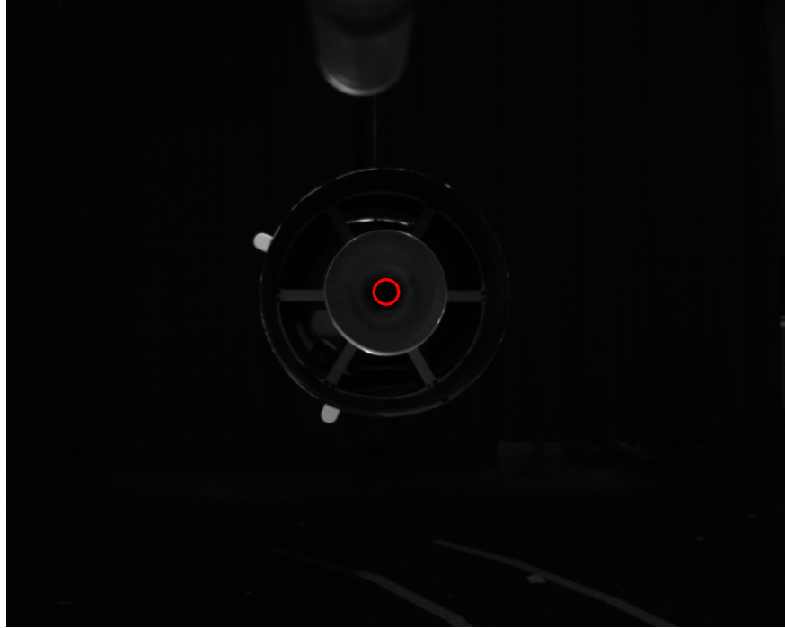
Figure 5.9: Image taken when the tracking algorithm determines target nozzle is inline with the camera. The red circle represents the location the projectile would be deployed.
