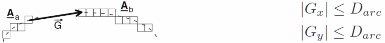
Figure 5.5: If two arcs are to be included in an elliptic arc, neither their horizontal nor their vertical distance may exceed D_{arc} [1].
