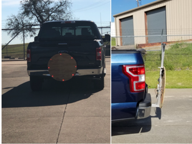
Figure 4.6: LED beacons set up for ground testing
