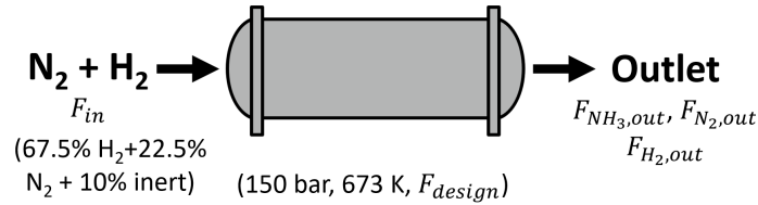
Figure G.4: Ammonia reactor input-output variables.
