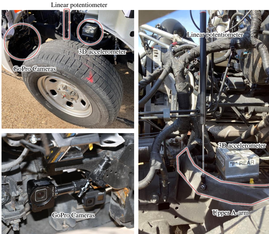
Figure 3.9 Instrumentation inside the left front wheel well (pickup truck)
