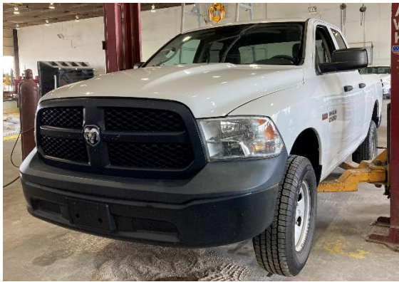
(b) 2270P test vehicle (before removing parts)
