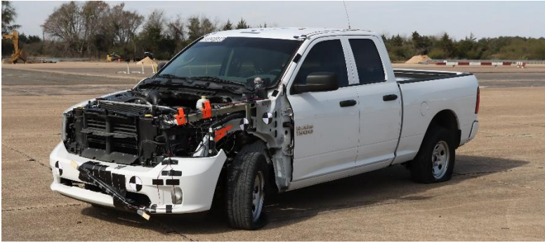
Figure 3.17 Pickup truck after the test
