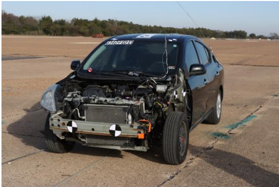
(c) 1100C test vehicle (after removing parts)
