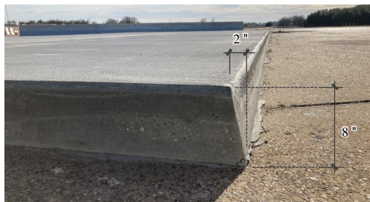
Figure 3.2 Profile of the test installation
