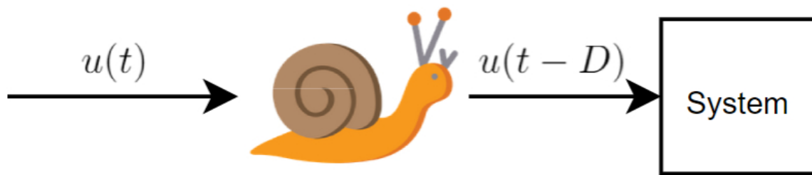
Figure 1.2: Time Delay in systems
