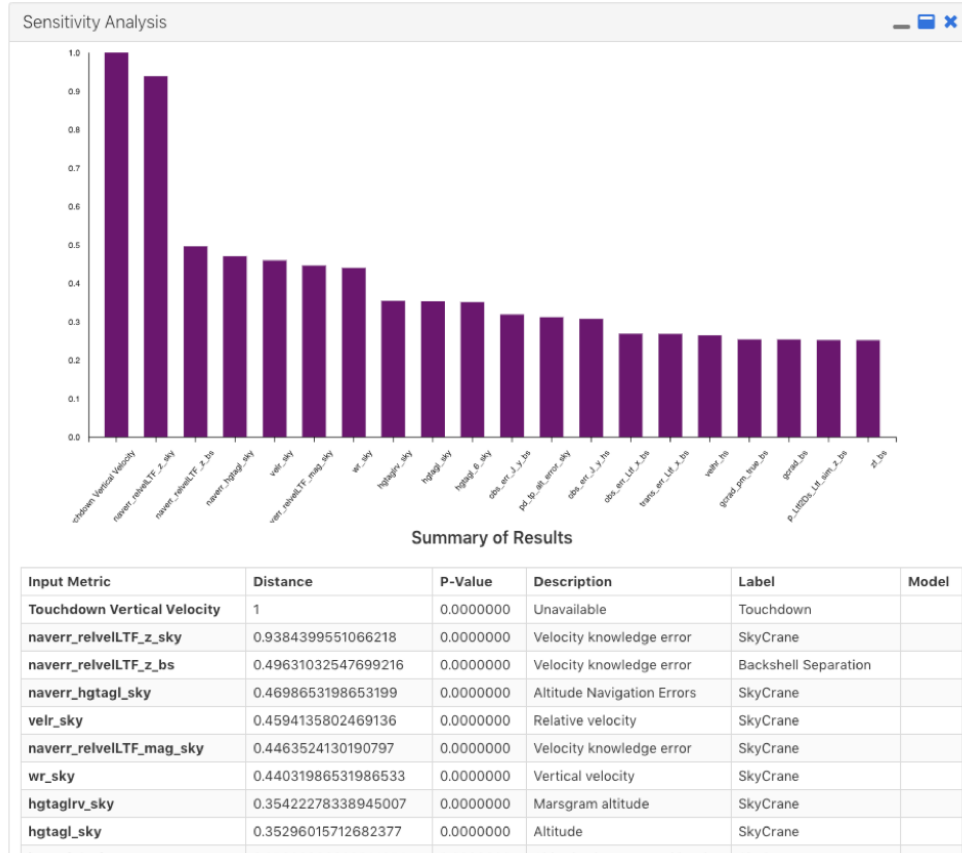
Figure 2.16: Results for a nadir-beam failure (Reprinted from [1]).
