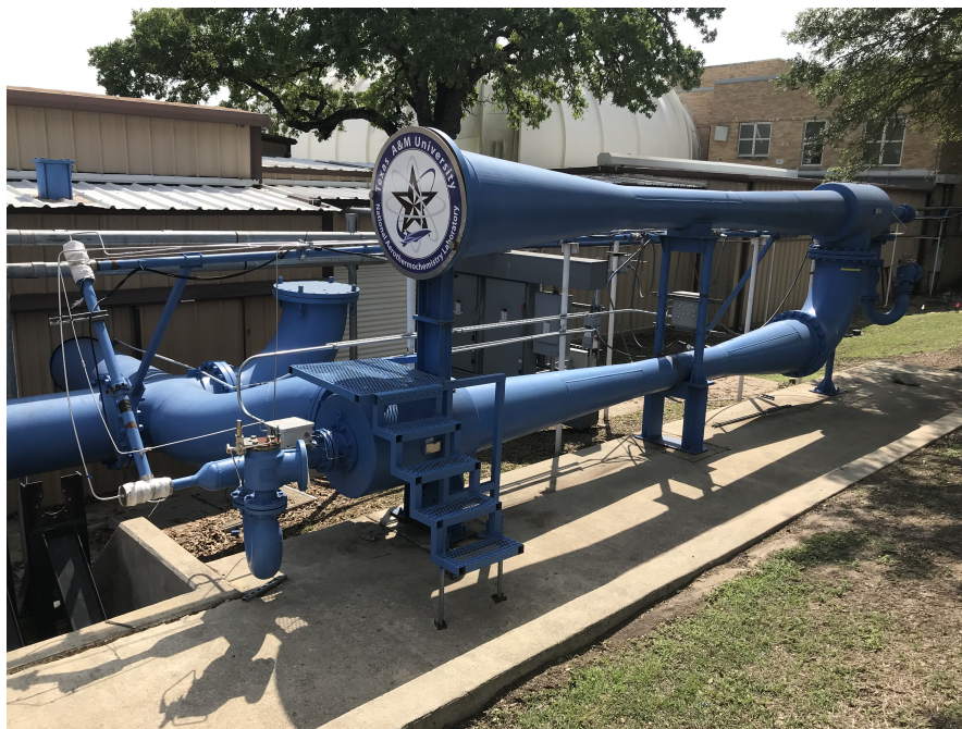
Figure 2.2: The two-stage Venturi air ejector that provides a vacuum on the downstream end of the blowdown wind tunnels.
