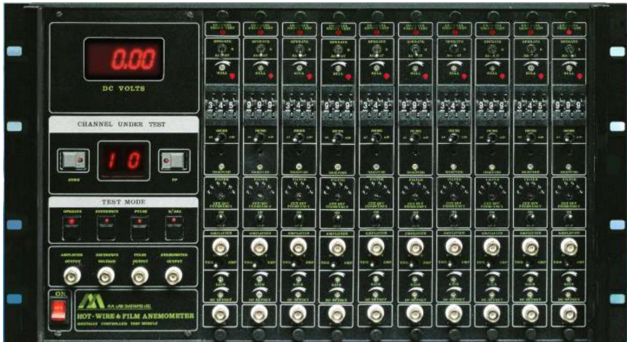
Figure 2.7: A.A. Lab Systems Inc. AN-1003 anemometer.
