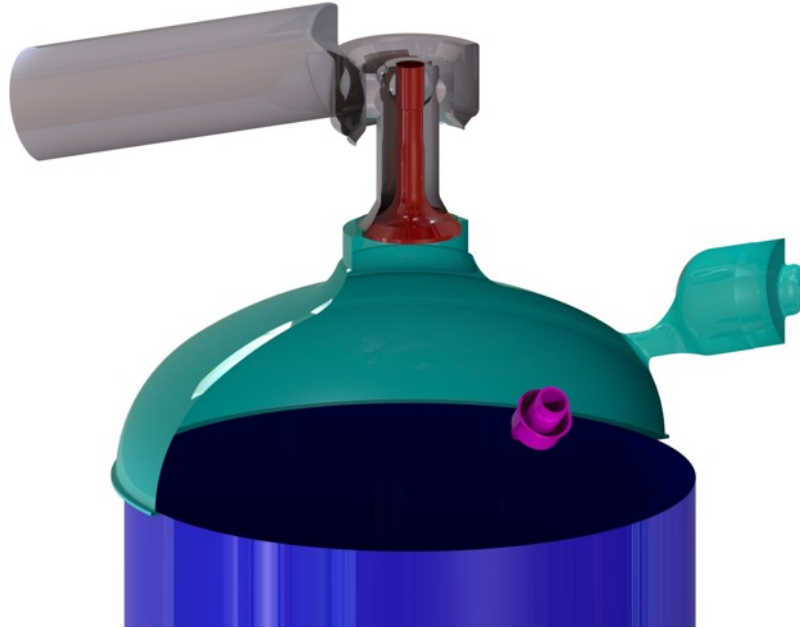
Figure 2.10: A cutaway view to show the interior of the added DI system geometry near the cylinder head, specifically the white housing and the maroon valve. The spark plug is purple and shown for relativity.
