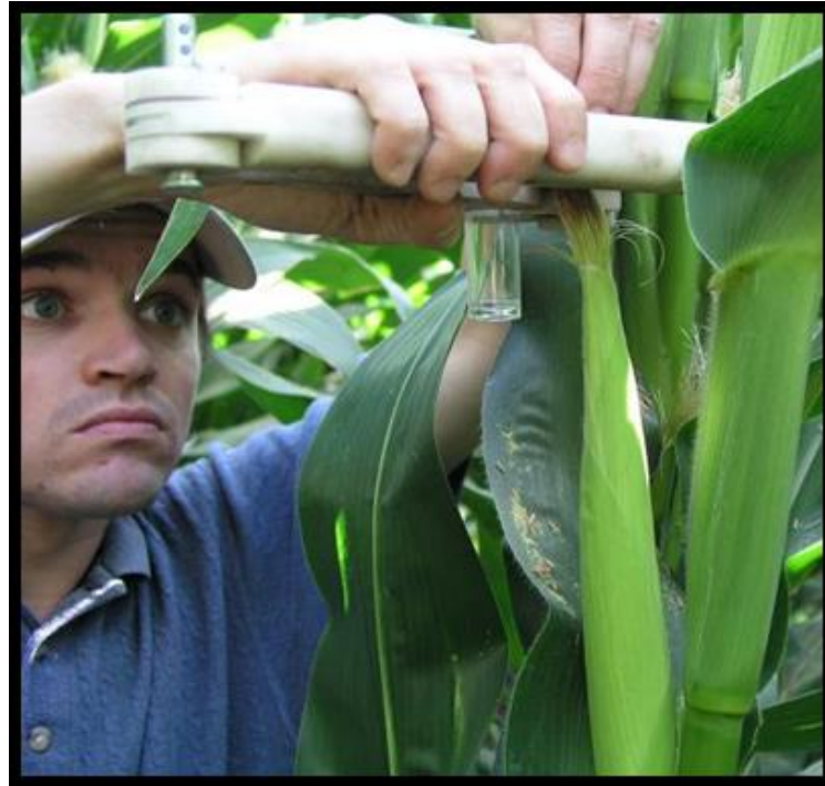
Figure 5: Utilizing the silk cutting device to harvest a silk sample
