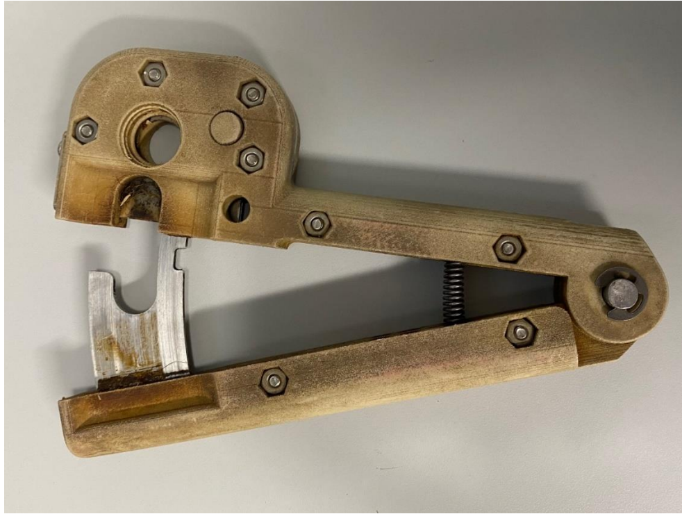
Figure 4: Silk cutting device developed by Corteva Agriscience
