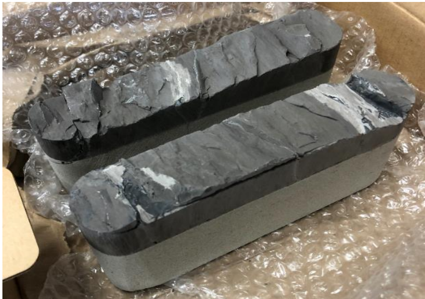
Figure 3-23: original fractured Austin chalk sample
