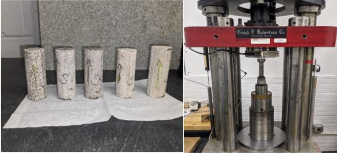
Figure 3-26: Core plugs for UCS (left), Large Sample Rig equipment for UCS (right)
