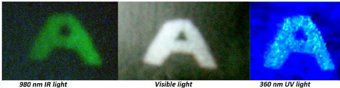
Figure 39. Images recorded by the constructed device under 980 nm IR, visible, and 360 nm UV light illumination. Reprinted with permission from (50).
