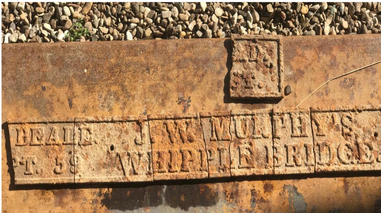
Figure 11. Beale Wagon Road's 1859 Whipple Iron Bridge Sign Bars Found Buried at Redbank Creek, near Spiro, Oklahoma, February 7, 2020, by Kyle Burch. The lower sign bar is 31"x 4"x 3/8" (inches).
