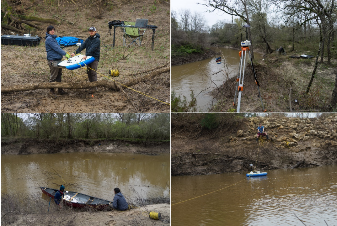
Figure 9. ADCP calibration by the river. Figure 10: Base station and control station in view of the canoe pulling the ADCP. Figure 11: Docking the canoe in preparation of transect data collection with a person on both banks of the river. Figure 12: Pulling the ADCP perpendicular of the channel banks to collect bathymetric and flow structure data.
