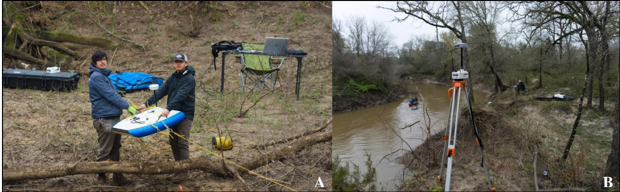
Figure 3. Field Instrumentation. (A) A Sontek M9 ADCP mounted on a Hydroboard was utilized during acoustic surveys. (B) An RTK-GPS Base Station was used to increase the spatial accuracy of ADCP data.
