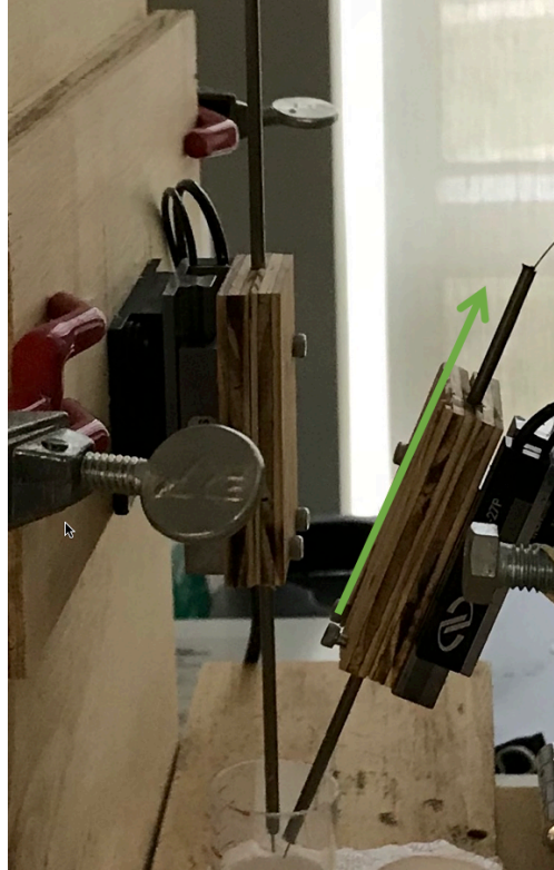
Figure 5. Demonstration of coordinate system used to control micromotor motion, with the green arrowhead indicating the direction of motion from positive values inputted for the “M1 Forward Step”, “M1 Backward Step”, “M2 Forward Step”, and “M2 Backward Step.”
