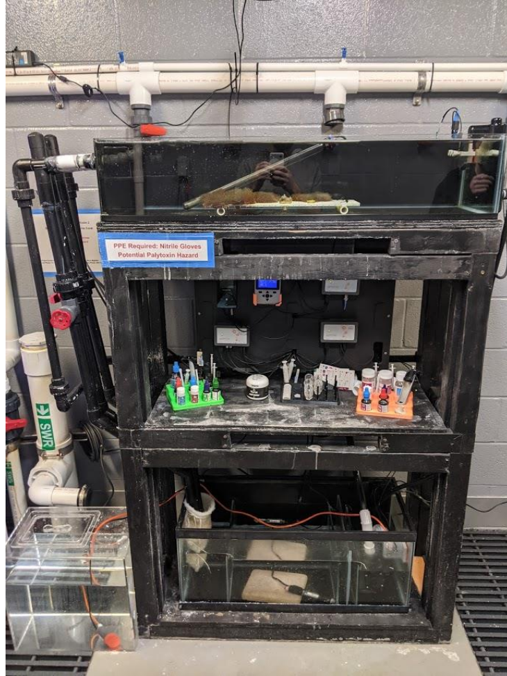
Figure 2.2: Coral tank set up. Top tank held the coral, probes, 300-watt heater, and UV sterilizer. Bottom middle tank is the sub tank. This tank held two 50-watt heaters, a sock, bio substrate and auto top off output. Left bottom tank was the top off tank that holds the auto top off intake.
