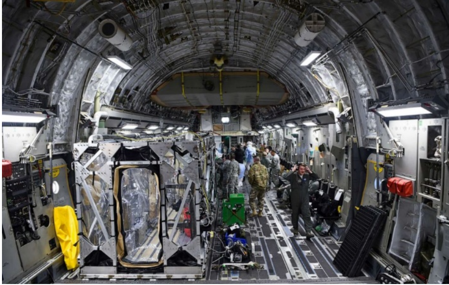
Figure 2.31: TIS interior isolation module and antechamber
