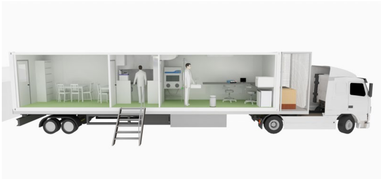
Figure 2.27: Mobile SURGE Conversion – Hospitainer Mobile Medical Unit
