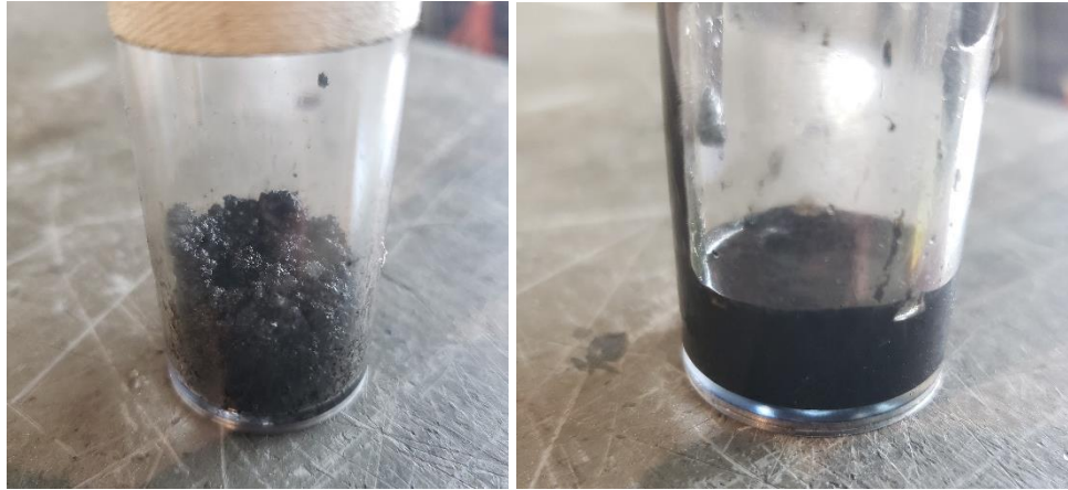
Figure 3.2: Collected deposits taken from test section for SAE 5W-30 conventional motor oil (left) and synthetic blend (right).
