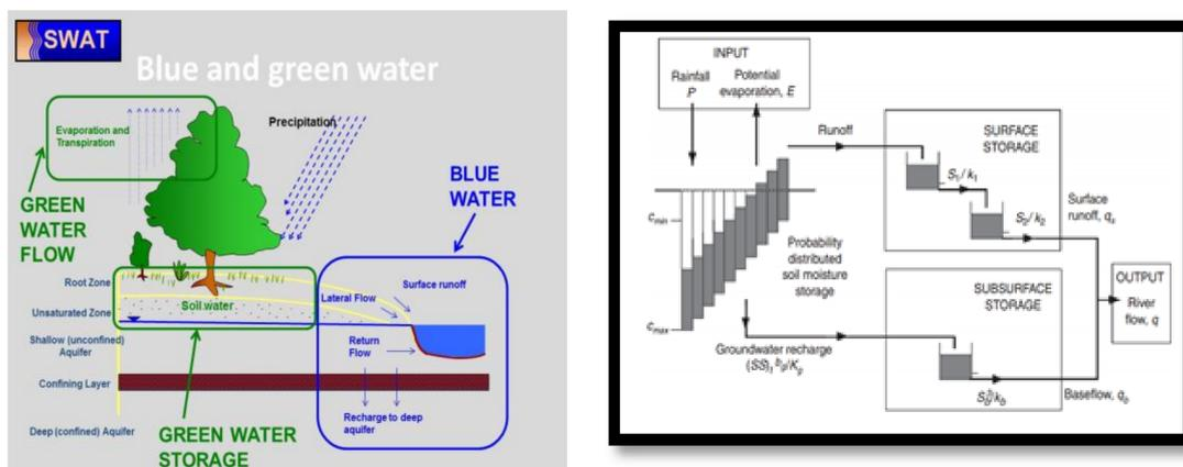
Figure 3. Schematic representation of SWAT [36] and PDM model (Source: Hydrology in Practice 2011).
