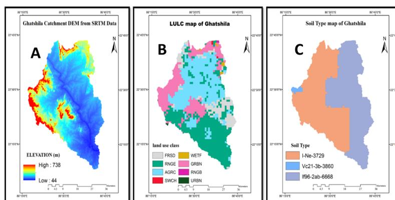
**Figure 2.** SWAT model inputs (A) Topography, (B) Land use/land cover, and (C) Soil type.
