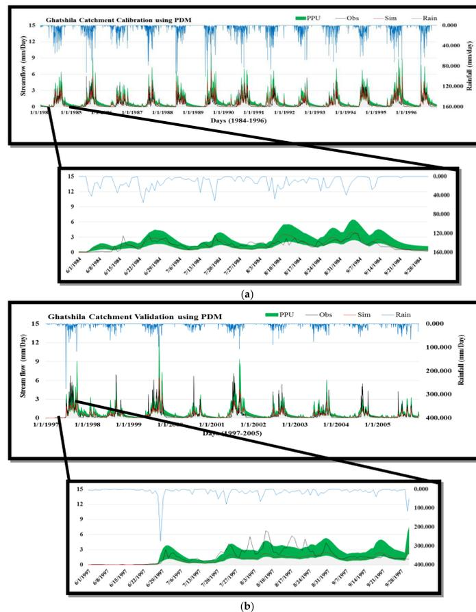
**Figure 6.** Comparison of simulated flow with observed flow of Ghatshila catchment. (a) Comparison of PDM simulated flow vs. observed flow (b) comparison of PDM simulated flow vs. observed flow.
