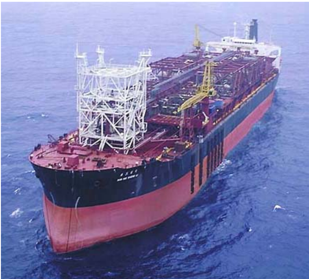
Figure 6. Floating, Production and Storage Offloading (FPSO)
