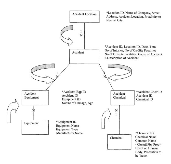
Figure 1. Database Model for Chemical Accident Information
