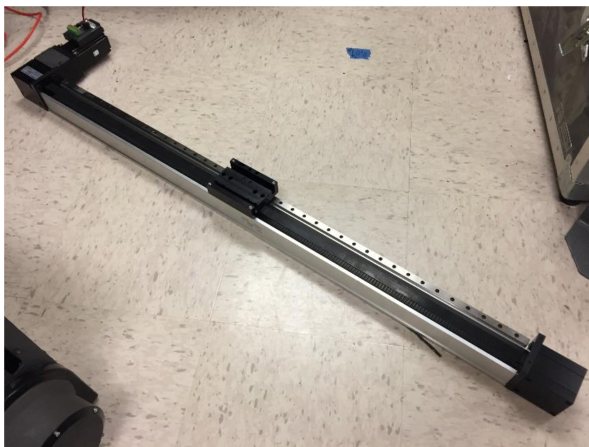
Figure 6. The 3-foot long linear actuator employed to move sources and detectors for the online laboratory.
