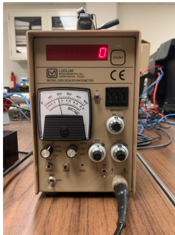
Figure 7. The Ludlum 2200 Scaler Ratemeter was used to control and take data from a GM detector.
