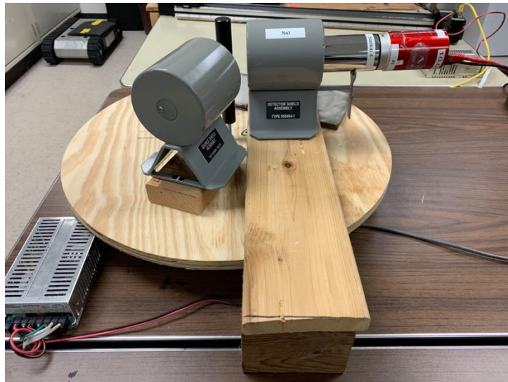
Figure 12. Apparatus of the Compton scattering experiment. The ^{137}\text{Cs} source is shown making a 70^\circ angle with the aluminum scattering rod.
