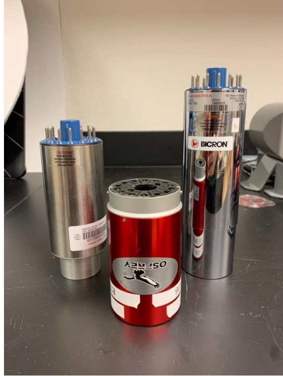
Figure 8. The Mirion Technologies Osprey™ MCA with LaBr (left) and NaI (right) detectors.
