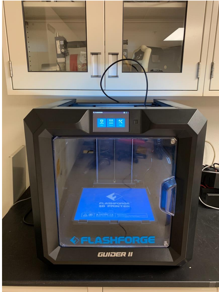
Figure 9. The FlashForge Guider II 3D Printer used to print source and equipment platforms.
