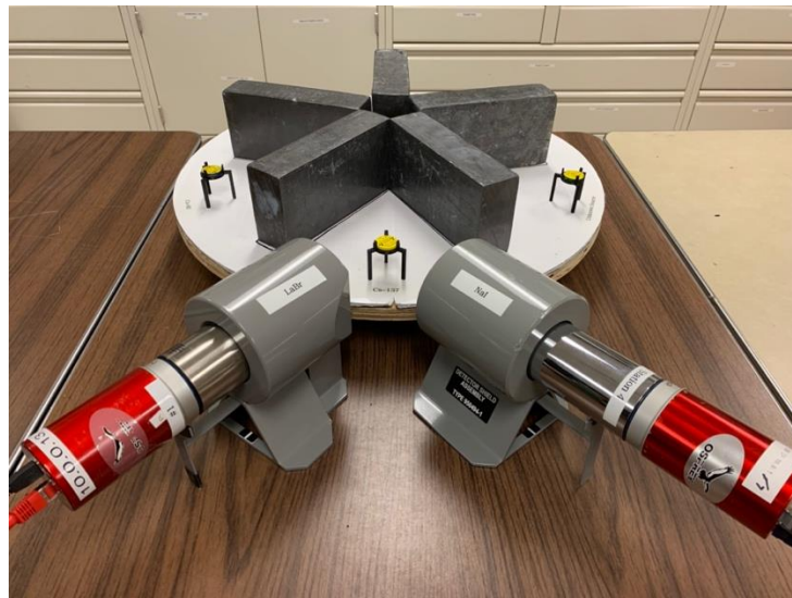
Figure 13. Apparatus of the spectroscopy with scintillation detectors experiment.
