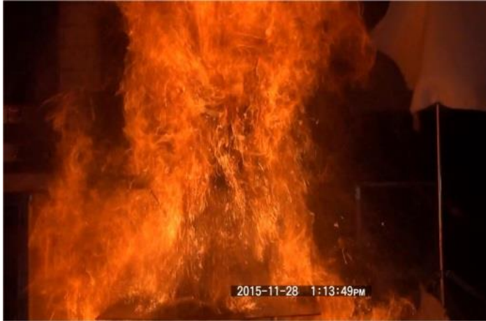
Figure 7 Example of photo of boilover (no bead, D=0.3m)
