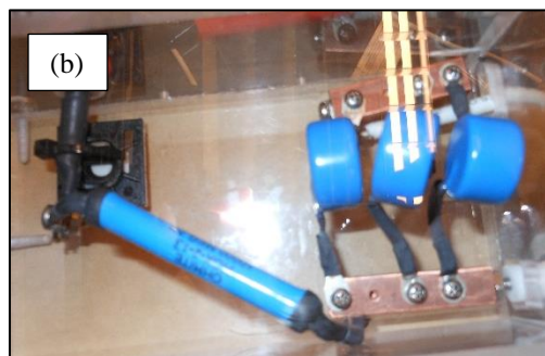
Figure 3. Minimum ignition energy (MIE) apparatus (a), custom-made by Fauske & Associates, that is used to determine the MIE of flammable gases. The amount of energy introduced to the flammable gas mixture is determined by the capacitance utilized (b).
