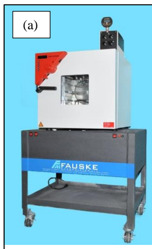
Figure 2. Flammability Chamber [(a) outside view and (b) glass test vessel], custom-made by Fauske & Associates, that is used to determine the lower and upper flammability limits and the limiting oxygen concentrations.
