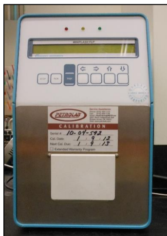
Figure 1. Miniflash automatic flash point (FP) tester (closed cup), purchased from Grabner Instruments, used to determine the FP of pure and diluted alcohols and alcohol mixtures.
