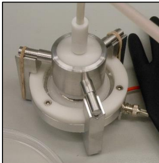
Figure 6. Powder volume resistivity apparatus purchased from Chilworth.
