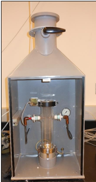
Figure 9. Modified Hartmann Tube Purchased from Adolf Kühner AG. This is used to obtain qualitative information about dust explosions.
