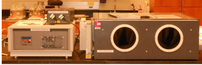
Figure 8. Humidity chamber purchased from Chilworth. This is used to control the humidity of electrostatic experiments that can be placed within the chamber.
