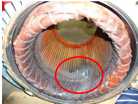
Figure 9. Insulation failure between layers of stator
