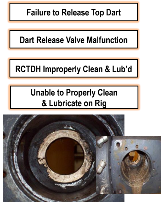
Figure 5. Typical investigation findings.
