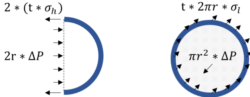
Figure 5. Simplified force balance around a cylindrical shell where a constant stress across the wall is assumed.
