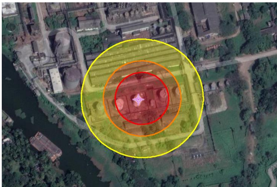
Figure 7 Thermal radiation footprint from Benzene Tank B
