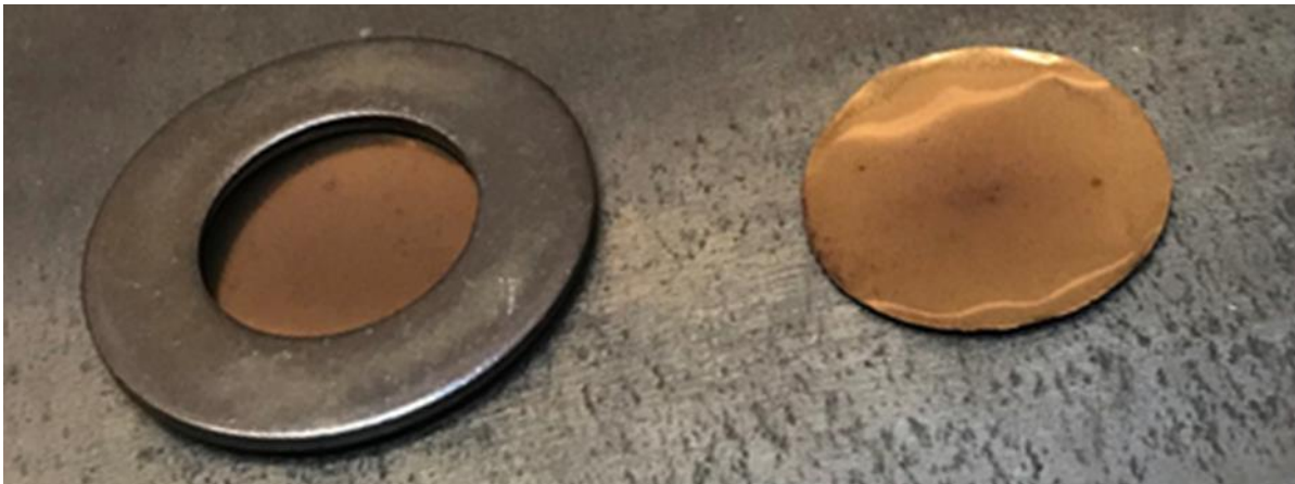
Figure 5. Second generation test surfaces. These are made from cut SS sheet metal and SS washers. Reprinted with permission from [16].
