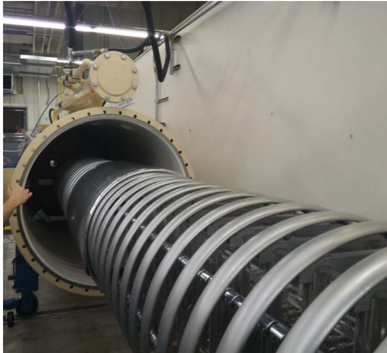
Figure 15 Inside the 3 MV accelerator pressure vessel, showing the terminal column at the center and the surrounding acceleration tubes.
