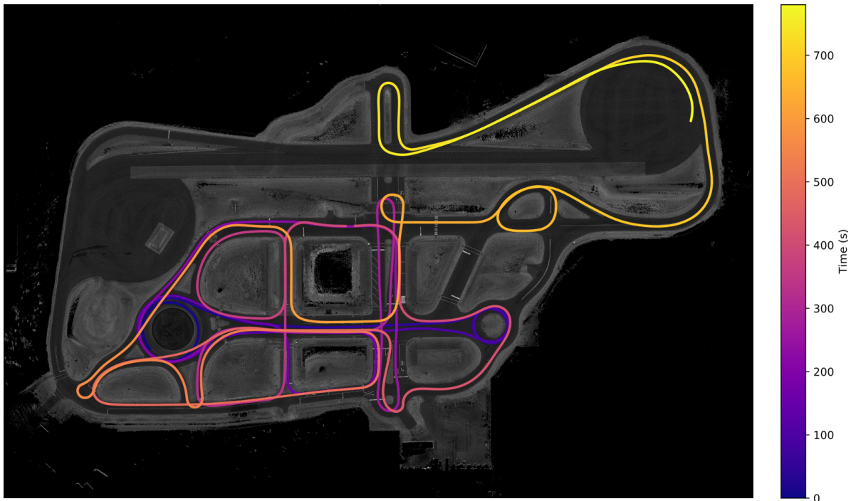
Figure 3.13: This figure shows the vehicle’s trajectory as calculated by our localization algorithm.
