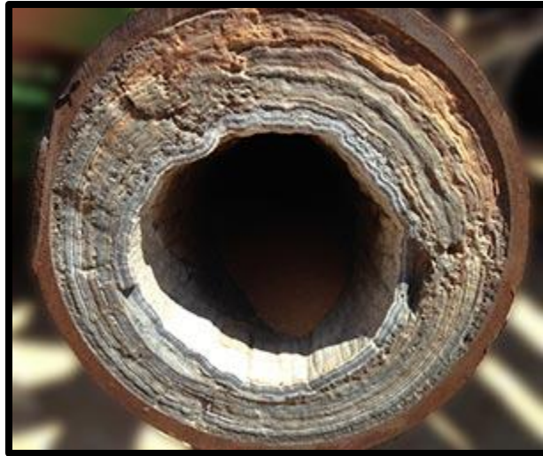
Fig. 1—Scale build-up in well tubulars.
